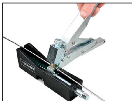
Cable lays into tool
