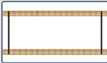
STEP #4 - Lay rails on a flat surface & install the two (2) outer balusters (four (4) screws per baluster). This will maintain spacing between rails.
