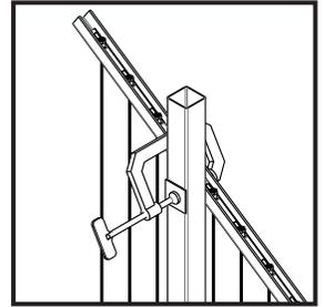
For Installations that span 24" to 60" a minimum of one Vertical Support is required. For installations 60" or greater two Vertical Supports are required.
