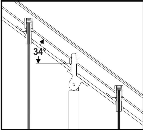
Vertical Cable Railing Stair Panels are designed with a nominal 34° of adjustability. The design allows for approximately 4° of adjustment in either direction. There will be a small amount of deflection in the cable at the stainless steel hardware.
