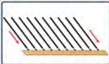
STEP #4 - Make sure connectors are properly lined up. Apply a small amount of silicone caulk to diameter of baluster where it meets baluster connector or insertion hole to insure a tight, movement-free installation. Install balusters on bottom rail.
