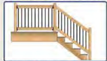
STEP #6 - Install stair rail assembly.
