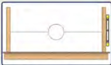
STEP #1 - Plumb posts/mounting surfaces. Measure inside distance of posts/mounting surfaces.
