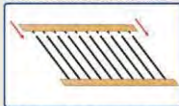
STEP #5 - Start Top Rail at an angle and insert connectors into balusters or into insertion holes until all balusters are in place. Make sure balusters are fully connected.
