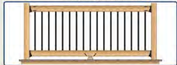
STEP #5 - Place top rail into position. Install four (4) #8 x 2" screws (per connector) through railing connectors into posts. NOTE: With spans greater than 6' (or required) install a foot block (use cut-off from rail).
