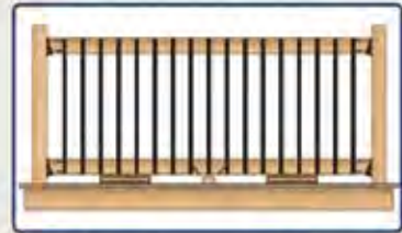
STEP #6 - Rest rail section on two (2) temporary spacer blocks the required height between deck and bottom of bottom rail. Center railing connectors on post and install four (4) #8 x 2" screws (per connector) through railing connector into posts. NOTE: With spans greater than 6' (or required), install a foot block (use cut-off from rail).
