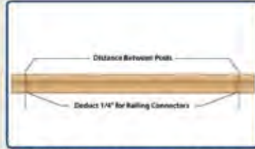
STEP #2 - Using step - 1 measurement, deduct 1/2" from total measurement for railing connectors (if not using railing connectors, cut to step - 1 measurement). Cut both top and bottom rails.
