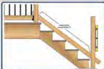
STEP #1 - Lay bottom rail alongside posts and mark for angle. If posts are plumb top rail should be the same length and angle. Cut top and bottom stair rails at proper angle.
