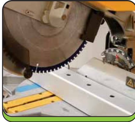
Step 11: Cut post at the marked cut line from Step 10. (Use a high tooth count metal cutting blade).
