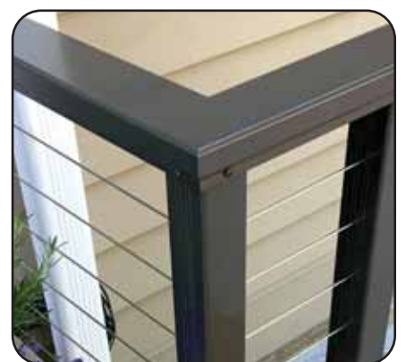
Single Corner Post - Application Once top rail is secured with a splice, it can be placed onto the post. Use 2 ea. screws to attach top rail to post.
