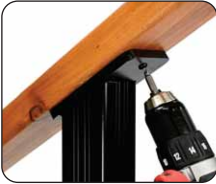
Stair Top Plate - Step 4 Wood top rail attaches to level top plate using 1 ea. screws from the bottom side. (Screw not included)
