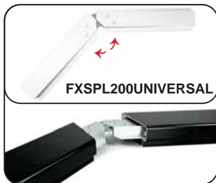
200 - Multi-Angle Splice - Step 1 Miter top rails to achieve the correct angle and slide splice into each end of the rail. Splice can accommodate angles between 0 - 90 Degrees
