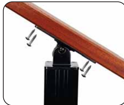
Adjustable Top Plate - Step 5 Wood cap rail attaches to Adjustable top plate using 4 ea. screws from the bottom side. Pre-drill if desired. (Screws not included)
