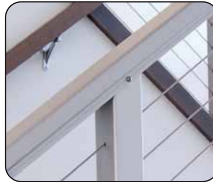
Series 200 Stair Intermediate Post Post must be cut at the angle of the stairs. Rail slides over top of post and attaches with 2 ea. screws. 1 screw on each side.
