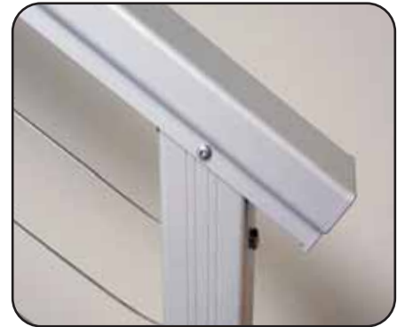
Series 200 Stair End Post Post must be cut at the angle of the stairs. Rail slides over top of post and attaches with 2 ea. screws. 1 screw on each side.
