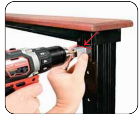
(3) Locate Rail Connecting Block (RCB) Align the RCB with the line made in Step 2 and center the RCB on the end plate bracket. Pre-drill the end plate bracket with 5/32" drill bit using the RCB as a guide.
