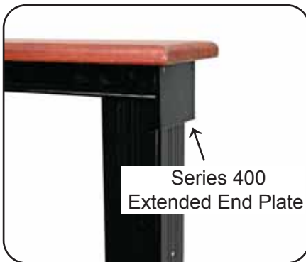
(1) Attach Extended End Plate Attach extended end plate to series 400 top rail using 2 ea. screws included. (Keep end plate tight to post)
