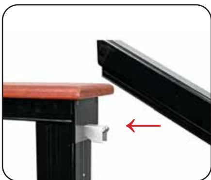
(8) Set Top Rail in Place Place top rail onto RCB bracket to ensure the cut and fit are correct.
