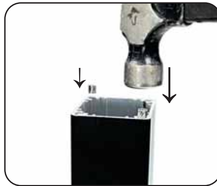
Adjustable Top Plate - Step 2 Tap 4 ea. screw inserts down into the post screw bosses using a hammer until flush with the post.
