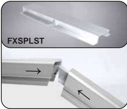
Series 200 - Stair Splice - Step 1 Miter top rails to accommodate stair angle. Bend splice to the correct angle of the stairs and slide splice into each end of the rail.
