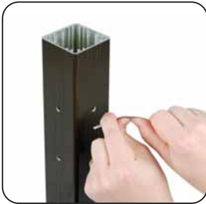
Step 1: Bend Cable Remove round tube from post. Create a slight bend in the cable to allow for cable to more easily pass through the single corner post.
