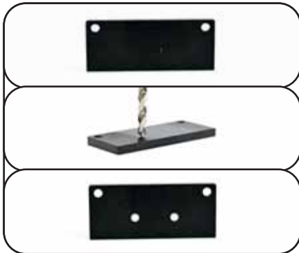
400 - Stair Splice - Step 1 Convert end plate into a bracket by drilling holes through the standard end plate.
