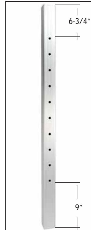
Stair End Post 2-3/8" X 45" Post - 10 Holes Item#: FXFMSCEP200XXX45 (29/64" Pre-Drilled Holes)
