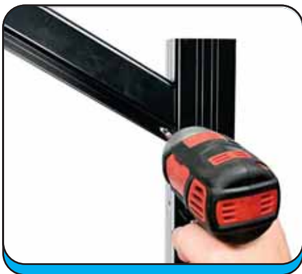
Step 17: Attach top rail to RCB using 1 screw on each side. Screws should be offset slightly to avoid colliding inside the rail.
