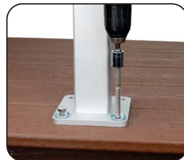
Step 3: Install cup washer under head of each fastener and drive fastener into blocking.
