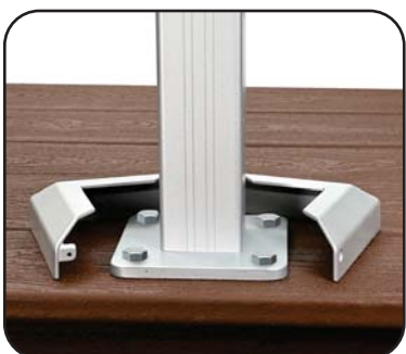
Step 6a: Install 2 piece post skirt. Secure with 2 screws (included)
