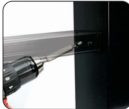
Series 400 Terminating into Post Step 2 Use 2 ea. included screws to attach end plate to top rail. Then use holes that were created to connect top rail into post or column.
