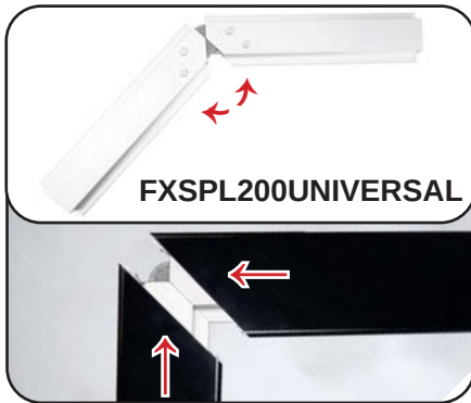
200 - 90 Degree Splice - Step 1 Miter top rails to create a 90 degree corner and slide splice into each end of the rail.
