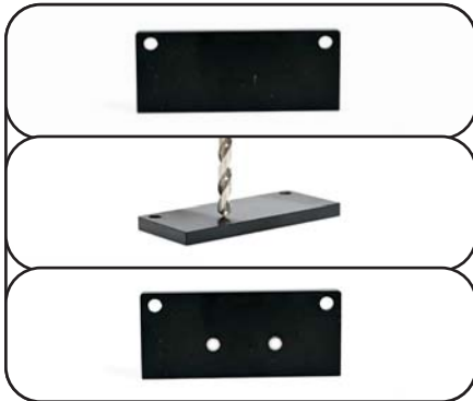
Series 400 Terminating into Post Step 1 Convert end plate into a bracket by drilling holes through the end plate for screws.
